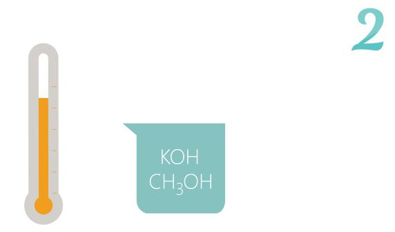
One method involves heating the vegetable oil in the presence of methanol and potassium hydroxide.
