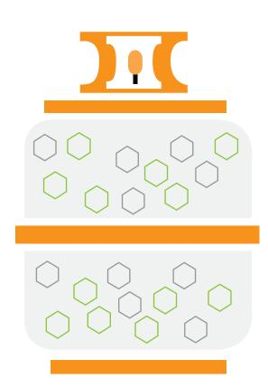
The mixture of fermentable sugars is placed in a tank with microbes. The sugars are converted into ethanol (see fermentation fact sheet).
