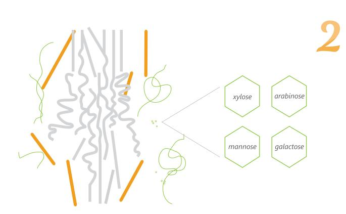
Before fermentation, plant biomass must be ground up and pre-treated with a hot dilute acid. This frees the cellulosic materials from the lignin and decomposes hemicellulose into its four individual sugars. Cellulose is still not broken down.
