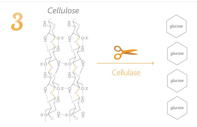
A process called cellulose hydrolysis deconstructs the cellulose. Sulfuric acid is washed off and enzymes called cellulases break down cellulose into individual glucose sugars.
