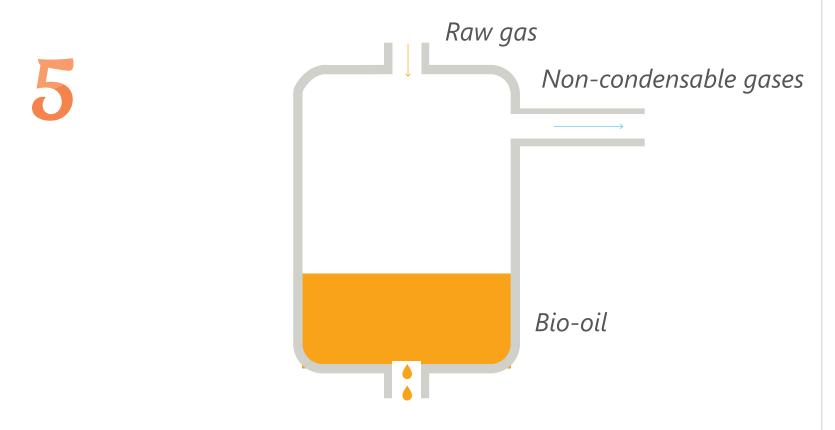
The raw gases are condensed into bio-oil. Non-condensable gases such as carbon monoxide can be recycled to fuel the pyrolysis reactor.
