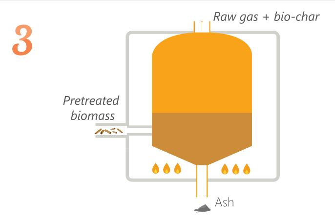
The biomass is subjected to high pressure and heat in an oxygen-free reactor. This produces solid bio-char, non-condensable gas, and gases that can be condensed into liquid bio-oil.
