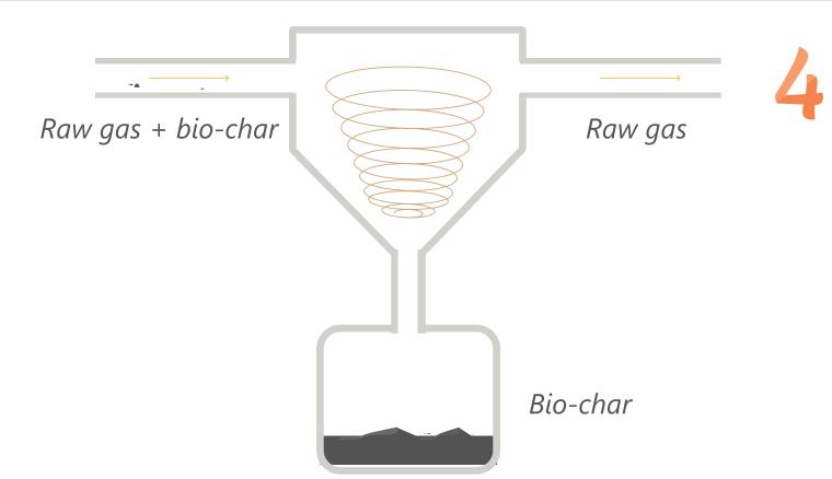
The solid bio-char is removed from the gases. Bio-char is a solid biofuel that can be burned to provide heat for the pyrolysis reactor or used as a replacement for coal.
