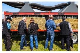
Figure 3. A new hay dryer (Ag Maximizer) design and built in Prince George BC and demonstrated at AgSmart. The heated air enters the baled hay through a series of vertical tubes penetrated into the large square bale. The sources of heated air is the heat recovery from a 375 hp diesel engine that runs the high pressure blower
